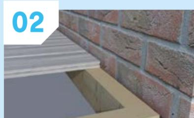
**02** 10mm between the wall and deck board.
