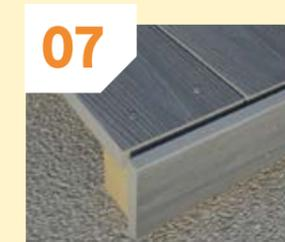
When using an Urban skirt trim across deck board ends, ensure the square edge is in line with the top surface of the Urban deck boards, check there is a 10mm gap between board ends and the vertical edge board.
