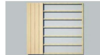
Each board should be supported by 3 joists. Ensure a slight fall of 2° to aid water run off.
